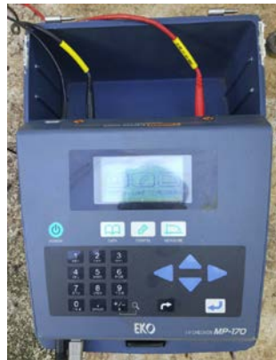
Figure 16 EKO MP-170 I-V curve checker
